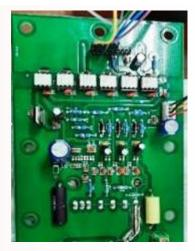
Fabricated circuit for re-phasing inverter
