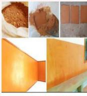
Developed soil-based wall care putty and applications
