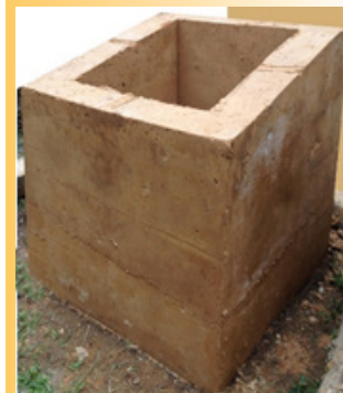
Prototype in-situ cast mud-concrete load-bearing wall model made for laboratory testing
