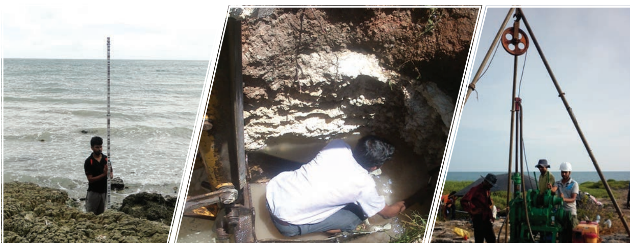
A - Measuring the height of the sampled in-situ coral heads; B - Studying buried corals at Polhena; C - Rotary core drilling of coral and limestone basement at Kachchativu Island
