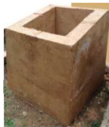
Prototype in-situ cast Mud-Concrete load-bearing wall models made for laboratory testing
