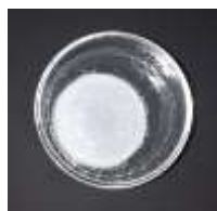
Figure 1: Ionic liquid based polymer electrolyte
