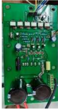
Fabricated circuit for re-phasing inverter
