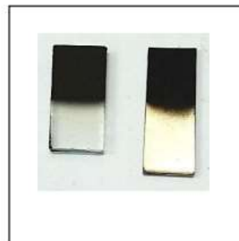
Counter electrodes for dye solar cells, prepared using activated carbon and sugar composite on conducting glass substrate and stainless-steel substrate
