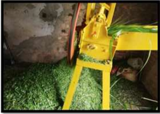
Figure 8: Chopping grass by grass chopper
