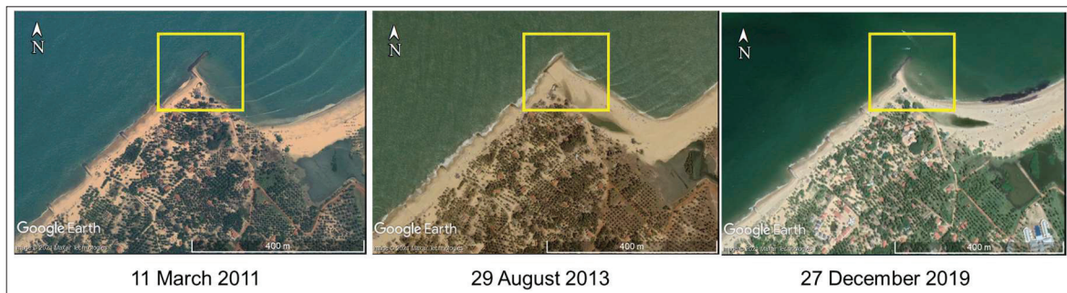
Figure 8: Satellite image photos of sediment accretion in the field of groynes on (a) 11 March 2011, (b) 29 August 2013 and (c) 27 December 2019
