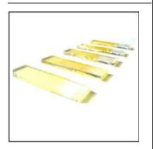
The fabricated chemical bath deposited CdS thin films
