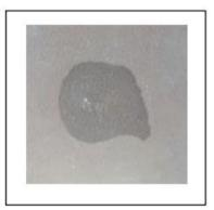
Gel polymer electrolyte hot pressed between two glass
