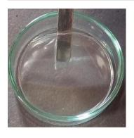
A gel polymer electrolyte prepared with solvent casting technique
