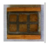
The fabricated CdS/CdTe solar cell
