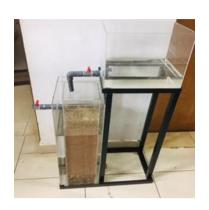
Lab scale filter unit which can be applied industrially
