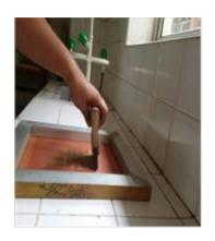
Fabrication of thin films using Screen Printing methods
