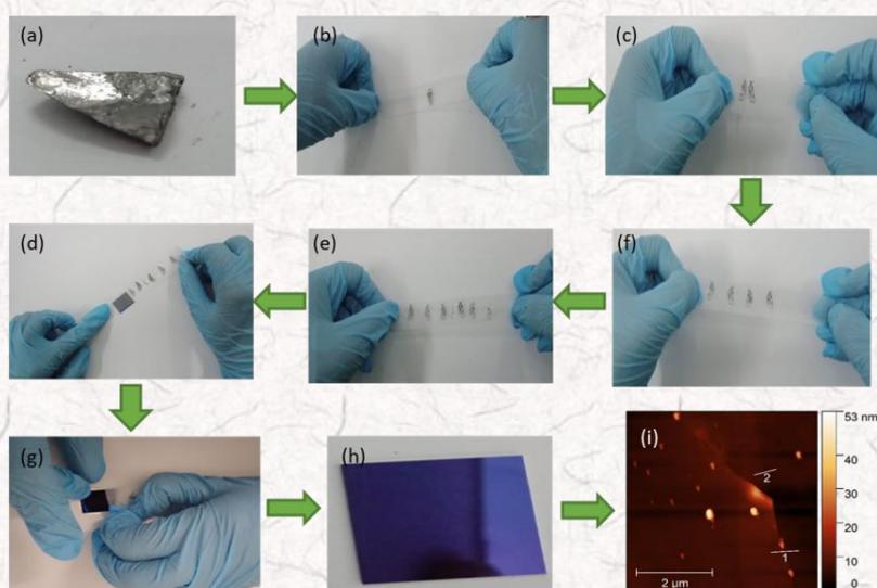
Extraction of graphene from a selected piece of graphite
