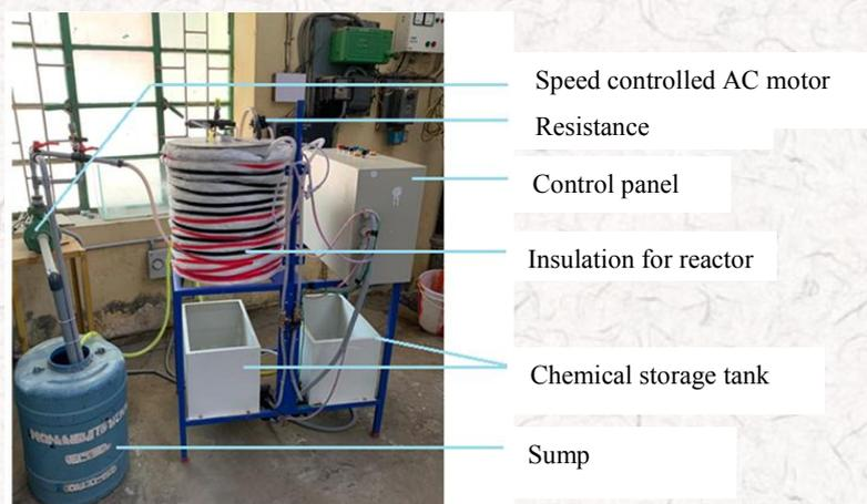
Experimental set up of continuous stirred tank reactors
