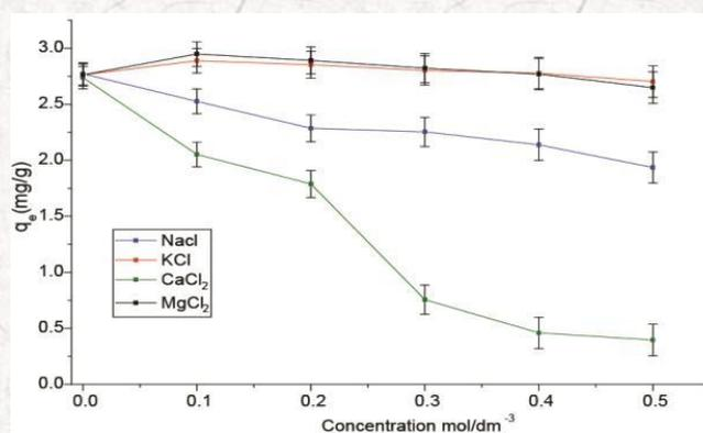
The effect of ionic strength on the MB removal efficiency
