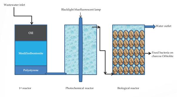
Schematic diagram of a full running coupled reactor
