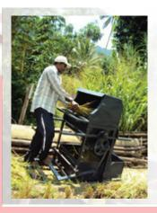
Paddle threshers are being used in Rice Research Institutes to thresh paddy during variety based research trials. Rice processing with the existing paddle threshers is strenuous, hard and paddy is not properly threshed. Further, it is difficult to maintain variety vise quality seed collection. The improved machine consists following features,
