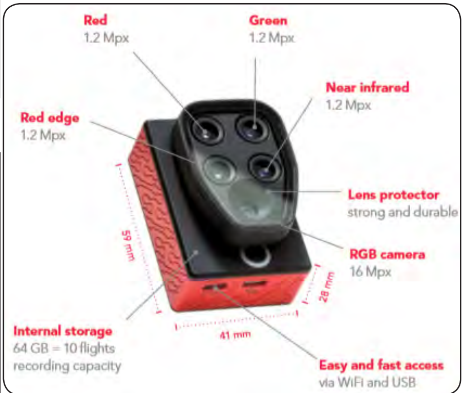
Fig 03 : Multi spectral drone camera (Green 550nm, Red 660nm, red-edge 735nm, Near Infra Red 790nm)
