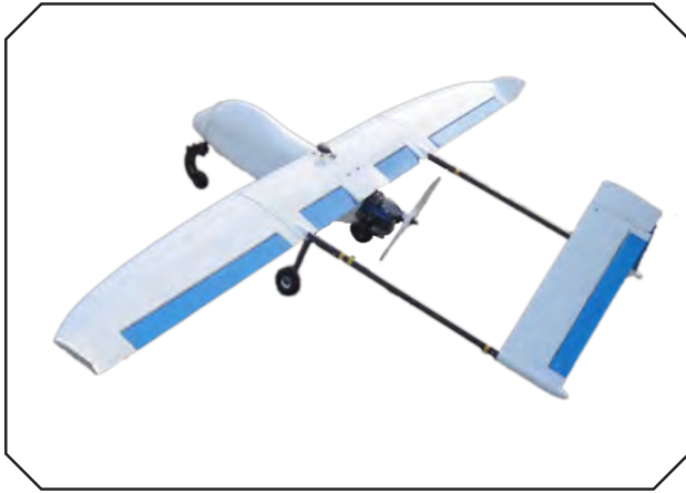
Fig 04: CeyHawk, 11kg engine powered long range drone developed at the University of Moratuwa
