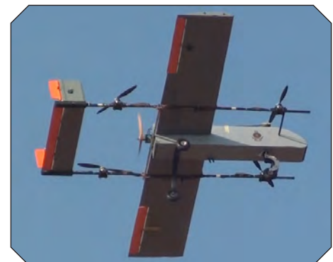
Fig 05: Hornet, quadrotor-wing hybrid drone of the University of Moratuwa (Funded by the National Research Council and the World Bank-AHEAD project)
